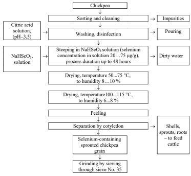
Fig. 2. Technological protocol for producing chickpea flour enriched with selenium
