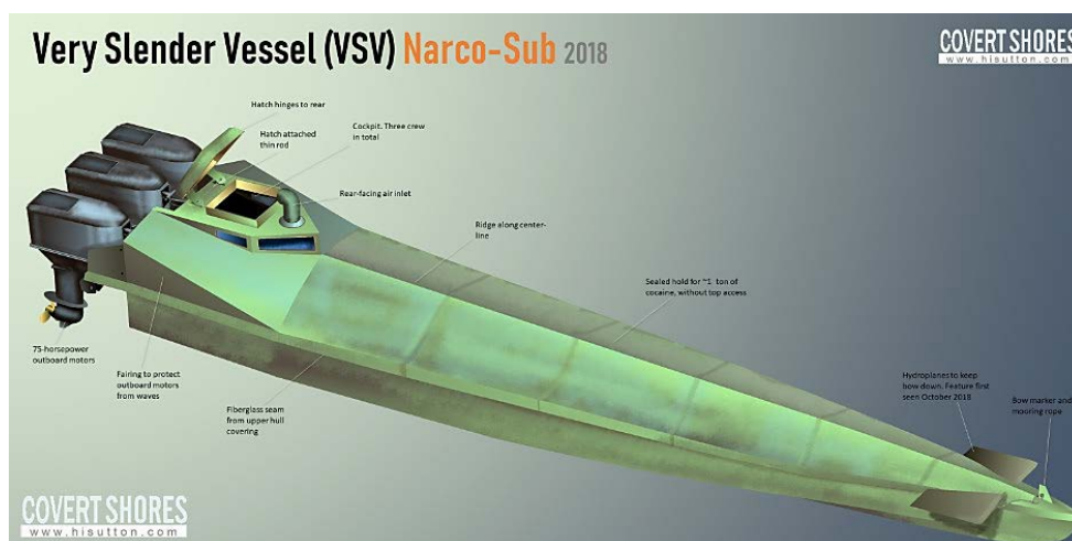
Figure 6. Very Slender Vessel (VSV) Narco-Submarine that is a low lying speed boat type that runs fast from South America to Middle America
